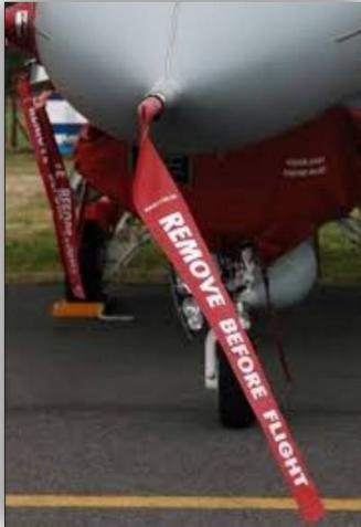
A simple, cheap and efficient system that allows operators and staff to know at all times that the pin is in place. As Spiecapag discussed with manufacturers and other contractors, this solution was never mentioned. This is an innovation.
