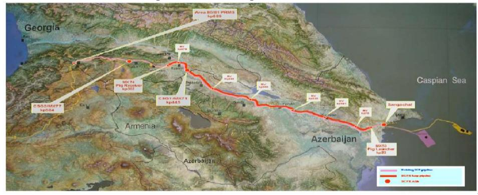
The expansion of the South Caucasus Pipeline is part of the Shah Deniz Full Field Development project. Expansion involves pipeline loop in Azerbaijan and shorter loop in Georgia along with two compressor stations. The new pipeline will be connected with TANAP at Georgian-Turkish border and will serve for further delivery of natural gas to European market through TAP. This will approximately triple the gas volumes exported through the pipeline to circa 23 bcma.
