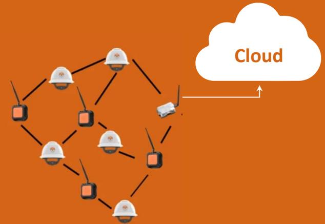
Nodes are placed across the jobsite to **expand connectivity** using a proprietary mesh network and to stream to the cloud via a gateway
