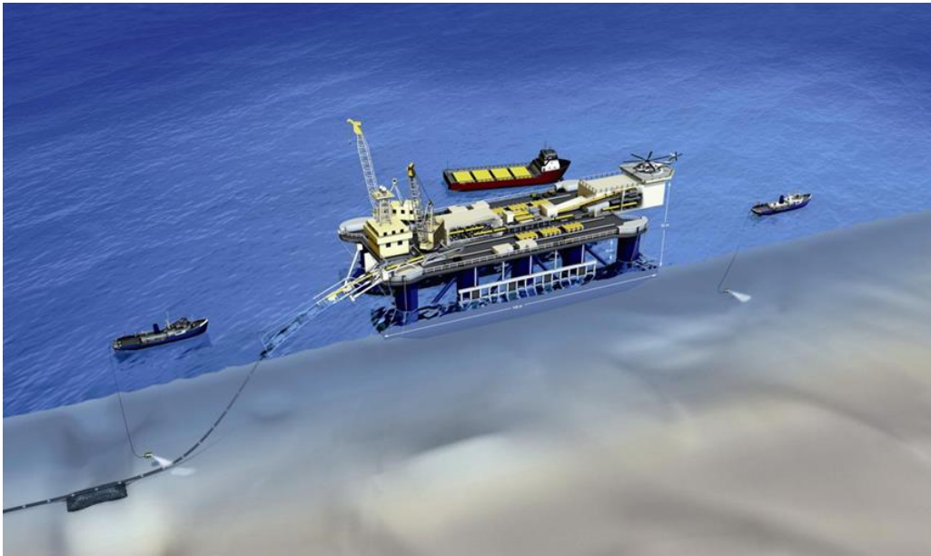
3D illustration of an offshore pipeline S-laying process
