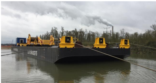
Figure 4-42 Winch pontoon (phase 1)
