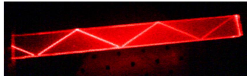
Total internal reflection on PMMA guide using a HeNe laser
