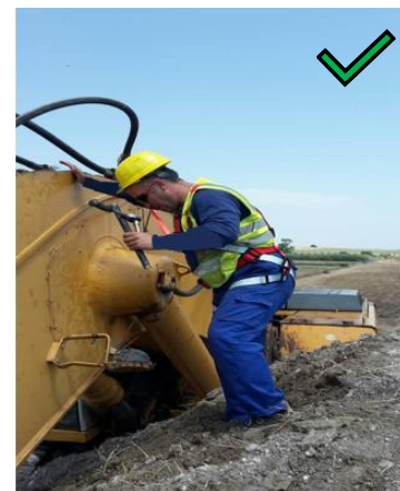
Fig 2. Correct method eliminating working at height
