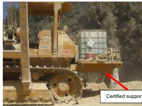
Fire-fighting equipment installed on our pipelayers.
