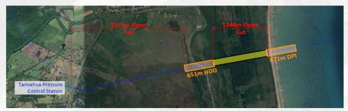
South landfall required 8 HDDs and a 670m 56" direct pipe installation completed by GDI and HDI
