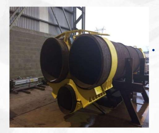
Bundle clamp for 2 NPS 42 pipelines and 1 NPS 24
