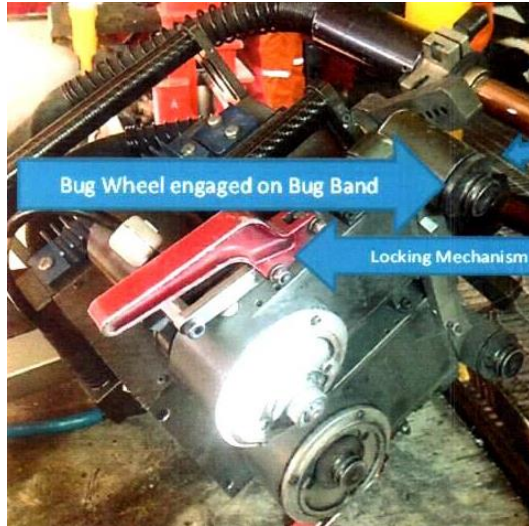
Locking mechanism on Bug, wasn't fully engaged.
