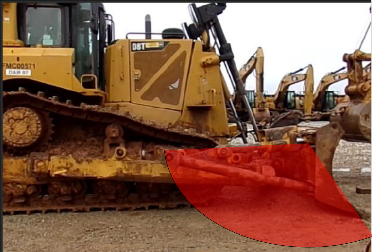
Danger Zone of A-frame
