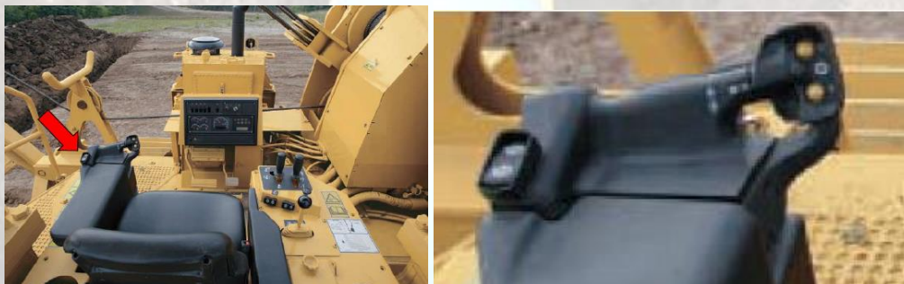
Picture 5: Plastic collar safeguard in place
