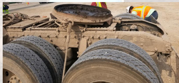
Picture 4: Failed Turntable
