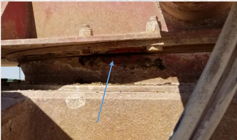
Picture 4: Vertical separation of top and bottom portions of turntable when lifted
