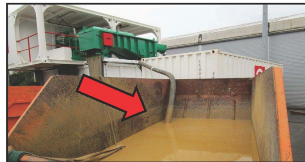
Untreated drilling fluid is pumped upwards.
