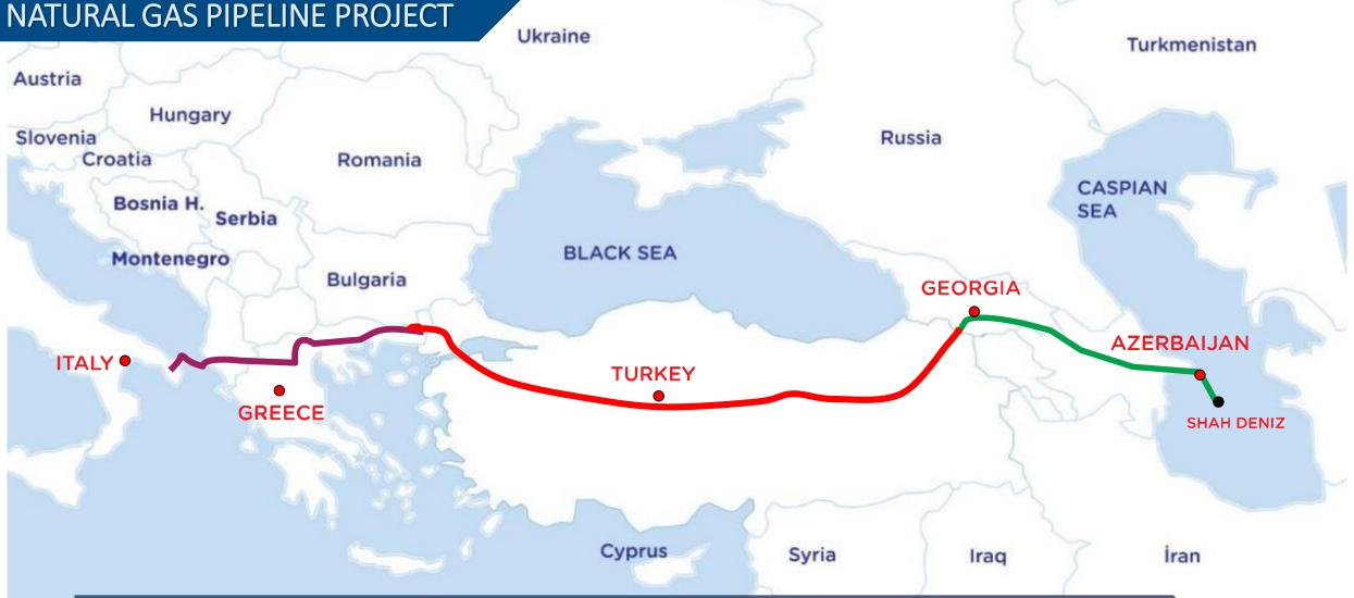
The TANAP starts from the Georgian-Turkish border where it connects to the South Caucasus Pipeline (SCP) and ends at the Turkish - Greek border, where it feeds into the Trans Adriatic Pipeline (TAP). There are two compressor stations and 4 metering stations on the line.
