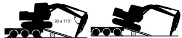
Example of loading and unloading of an excavator.
