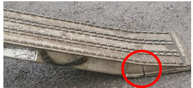
Damaged ramp identified before the unloading.
