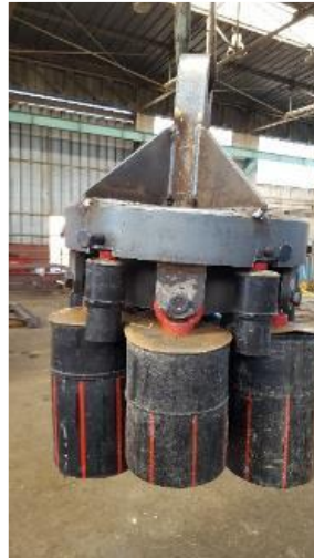
Lines fixed to pullhead
