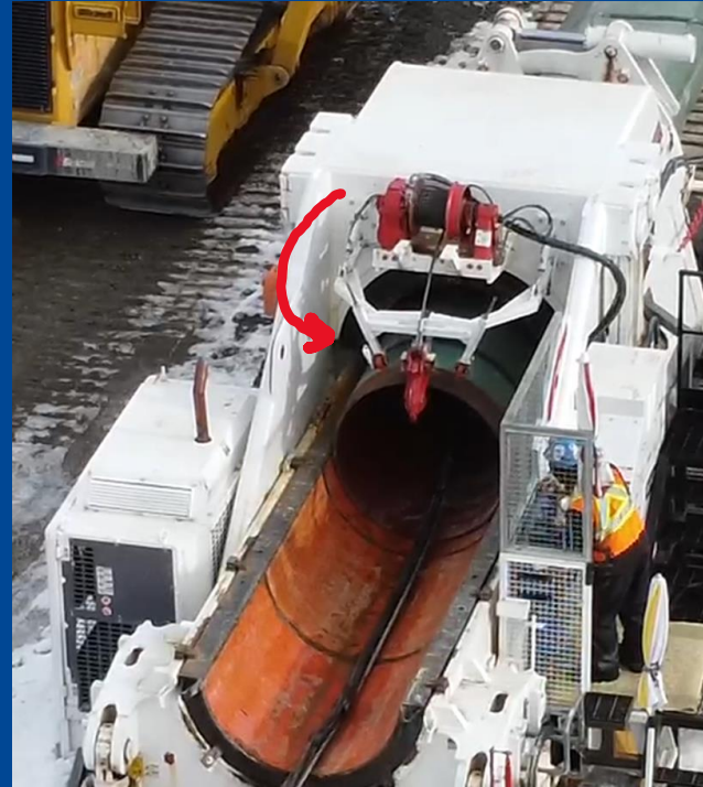
While pipe slides in, the support contacts the pipe, and the hook is positioned at optimal height to be attached to the bevel
