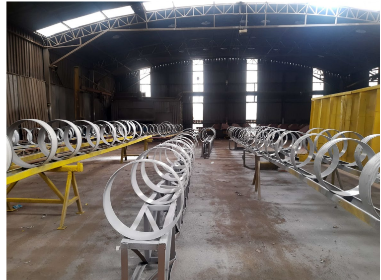
FlexSleeve coating is shop-applied and quality inspected before the welding even begins.
