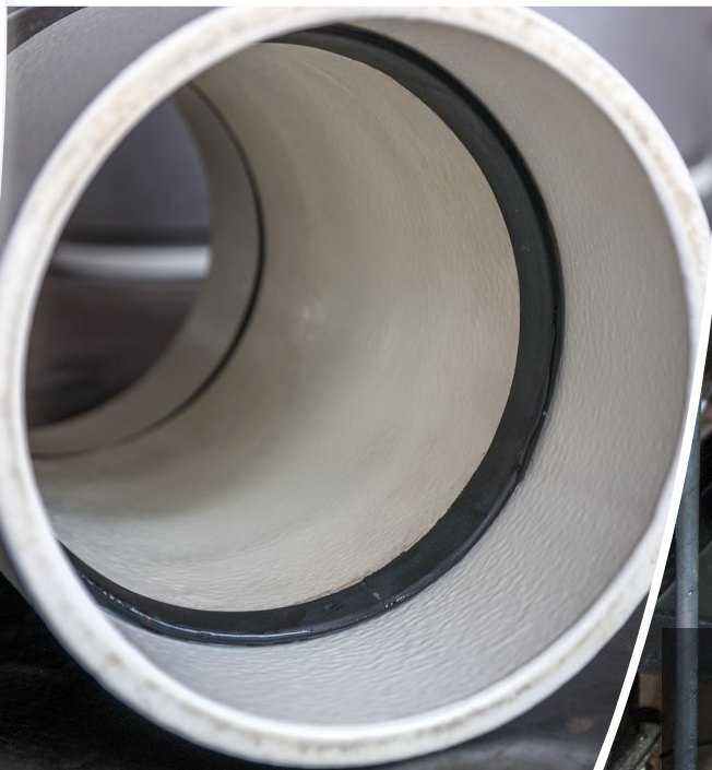
Hydrostatic pressure test with 6" dia. sch. 80 pipe without any weld
