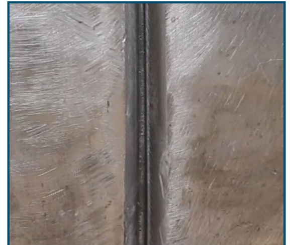
Set Weld Gap (V-Bevel)
