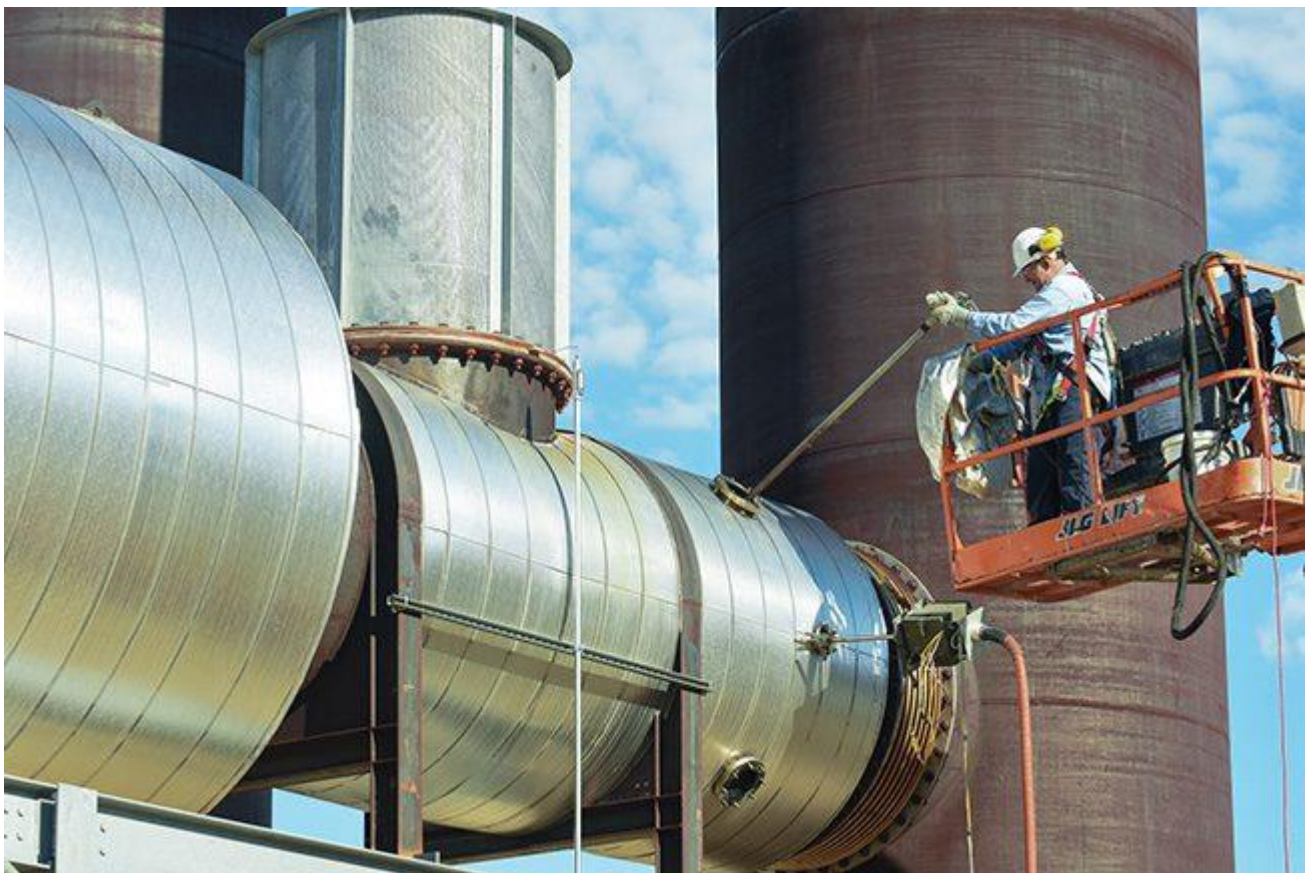
1. This worker is using a testing wand to collect measurements and other data as part of the hydrogen blending project at the A.J. Mihm facility. Courtesy: WEC Energy Group
