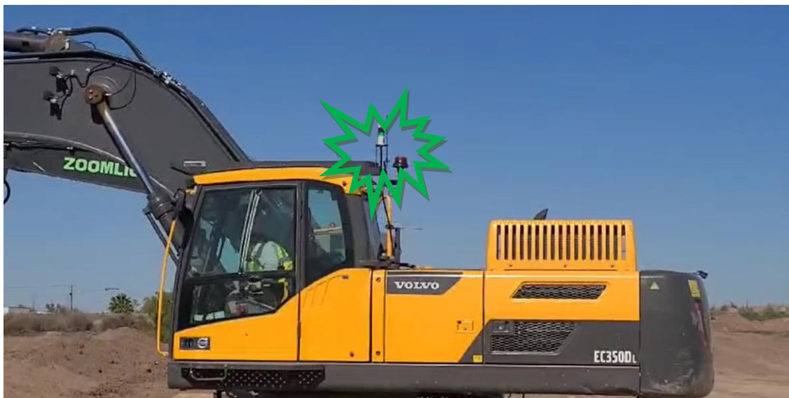
Green light when equipment is in stand-by
