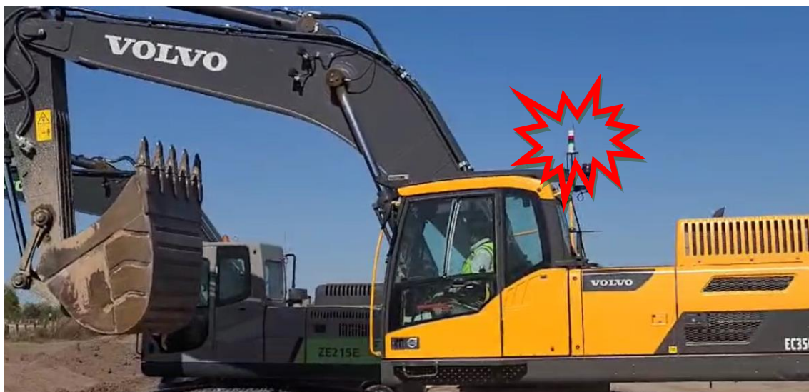
Red light with running equipment
