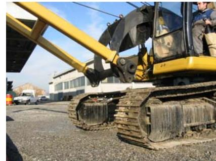
4. In the transport position, the upper structure is aligned with the undercarriage and the Sideboom Kit can be lowered for loading the machine onto a truck.
