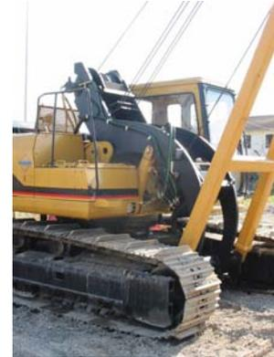
2. The structure also supports a pipelayer-type Sideboom. The original hydraulic system is maintained, with only slight modifications. This way, the operator can use the Sideboom functions with the original joy sticks of the machine.
