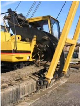
3. In the working position, the upper structure is rotated by 90 degrees and the Kit structure sits directly on the undercarriage, hence transferring the loads directly into the ground.
