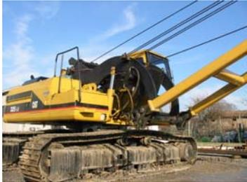
1. A main structure is installed in place of the original boom, using the same pins. This structure supports the two hydraulic winches that drive the boom and the block of the hoisting hook.
