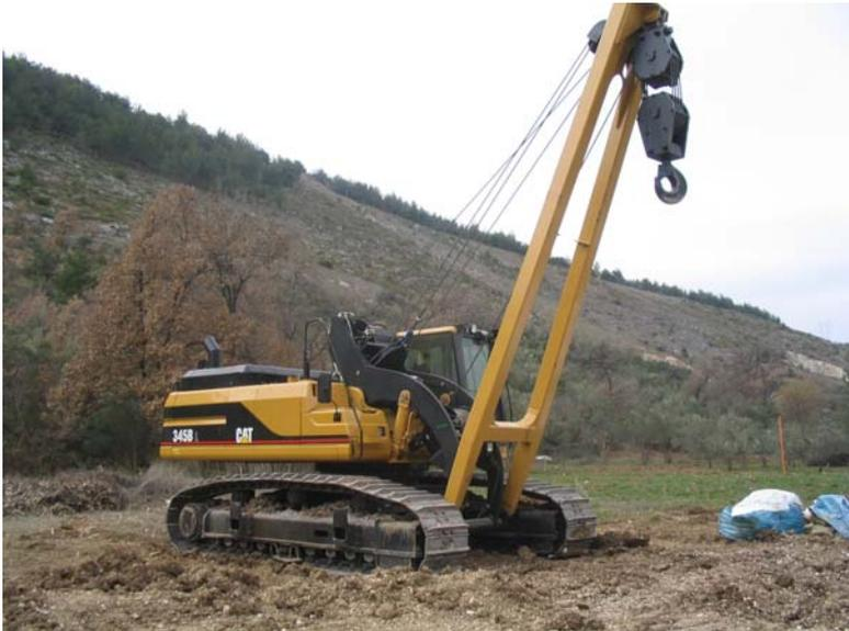
When used in confined areas or on tie-ins, or when mobility of equipment is a requirement and job-sites present features such as electric power lines or bridges, the use of the traditional Pipelayer becomes awkward and unpractical.
